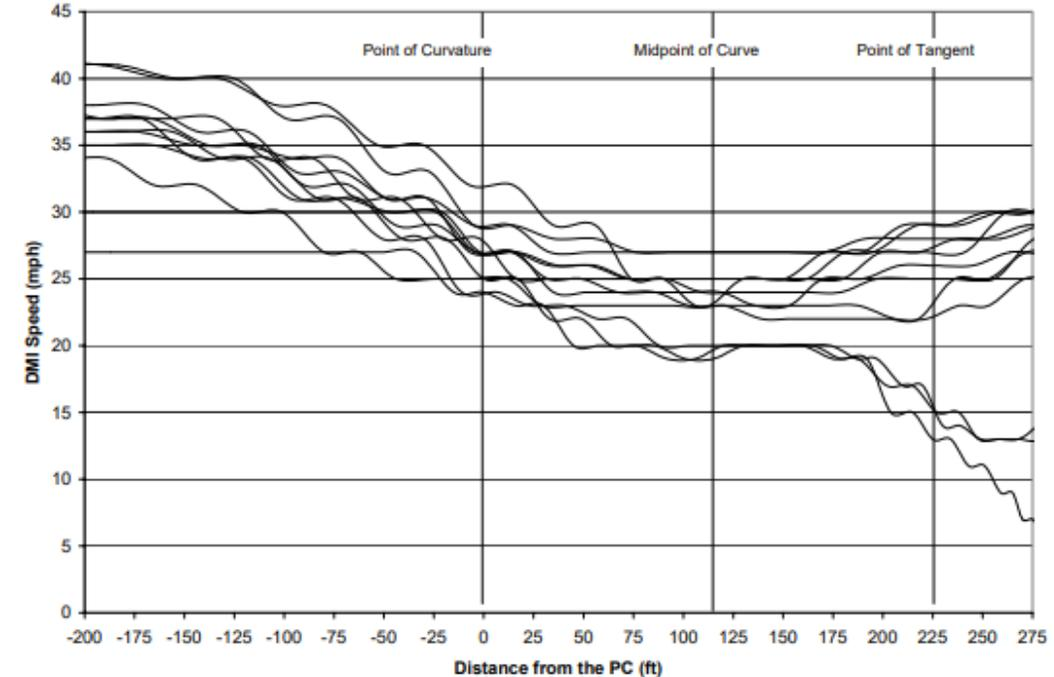
Figure 15. DMI Vehicle Speed Through Right Turn at Site 2.
