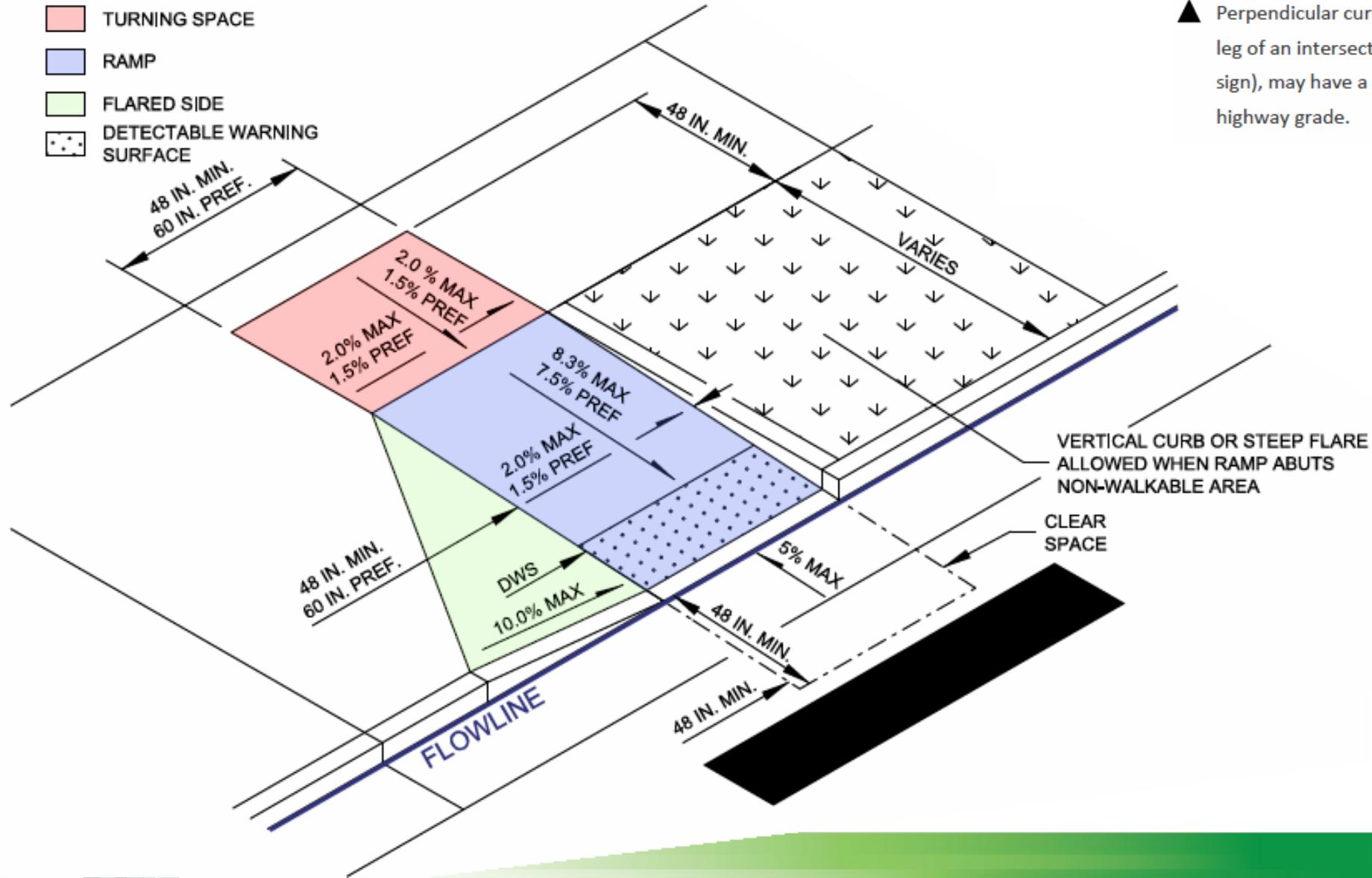
▲ Perpendicular curb ramps at a mid-block crossing, or crossing a leg of an intersection without stop control (yield sign, or stop sign), may have a ramp and turning space that equal the highway grade.
