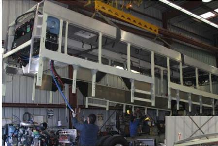
Structures are joined to make the bus frame
